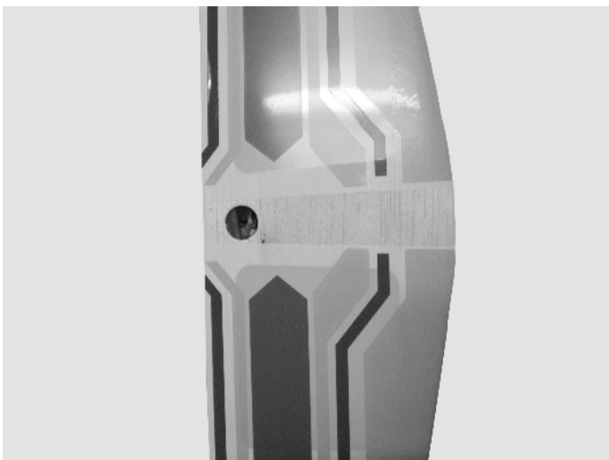
Put out the lightning connector through the hole in elevators upper side.
