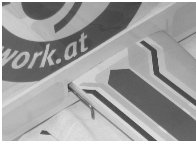
The connection bracket should be sanded at the glueing areas. Degrease it with brake cleaner. Insert the bracket into the fuselage.
